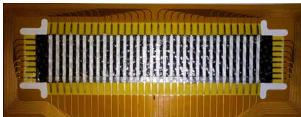
Figure 4: Photograph of flex-frame with FFRP sample
