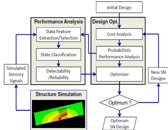
Figure 2: Flowchart of Detectability-Based Design Optimization Framework for Structural SN Design
