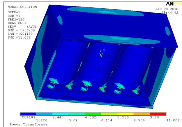
Figure 5: Stress Contour of the Winding Support for the Healthy State of Power Transformer
