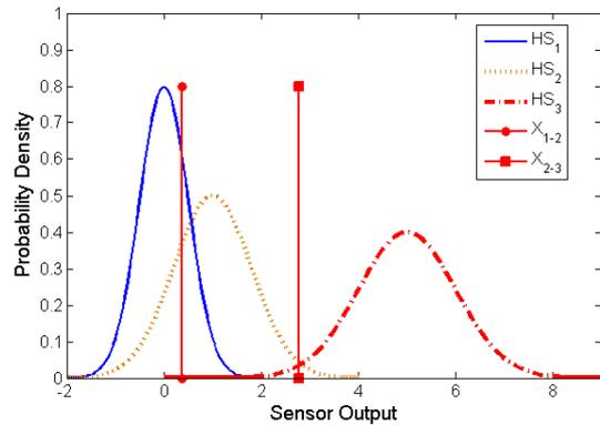
Figure 1: Sensor Outputs and Neutral Points between Health States
