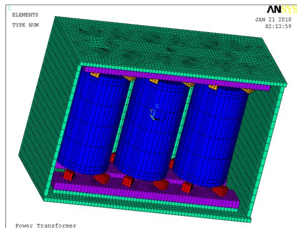
Figure 3: A Power Transformer FE Model (without the covering wall)
