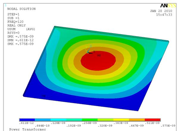
Figure 6: Vibration Displacement Contour of the Power Transformer Covering Wall for the Healthy State of Power Transformer
