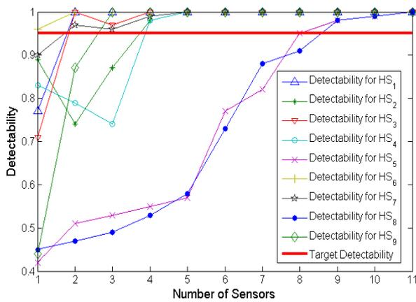
Figure 7: Minimum Detectability at Optimum Design versus Total Number of Sensors
