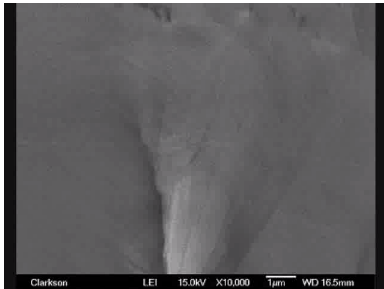
Crack growth during loading
