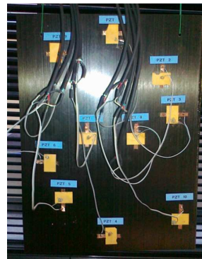
Figure 2 Healthy composite plate bonded with ten PZT patches
