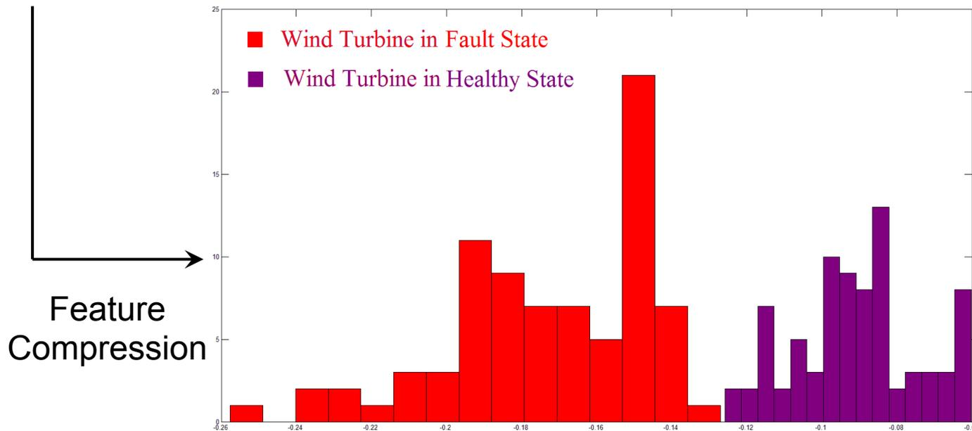
Figure The histogram of the transformed feature of the healthy machine and the machine with damaged components
