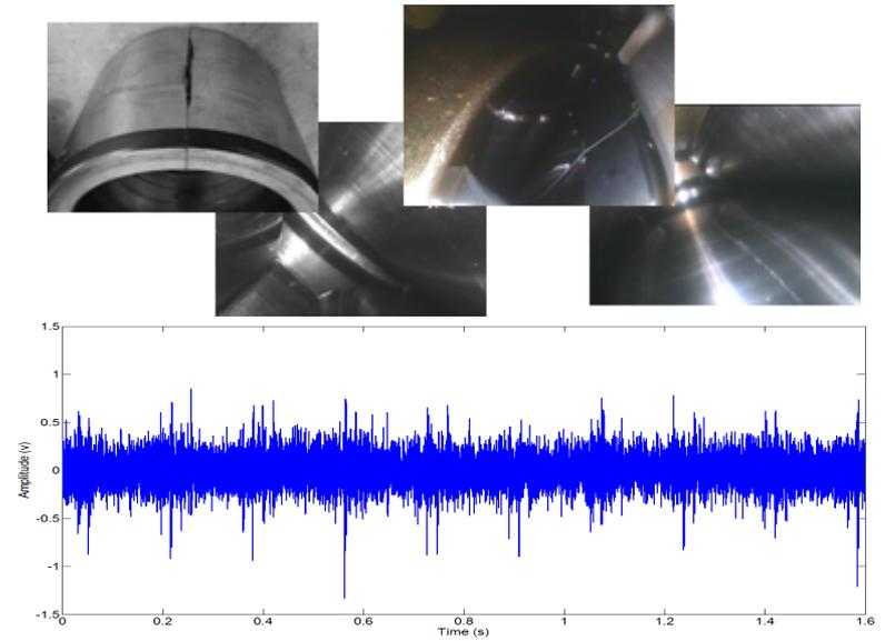
Signal of the gearbox with bearing inner race defect
