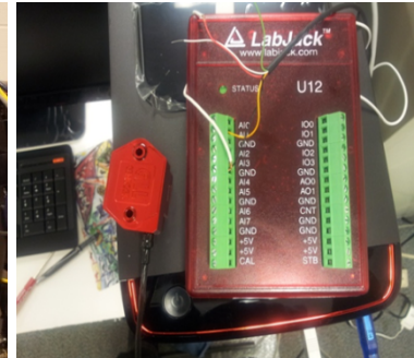
Dielectric constant sensor and the LabJack U12 data acquisition system
