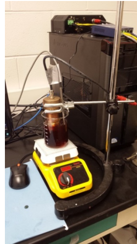
Dielectric constant sensor and the LabJack U12 data acquisition system
