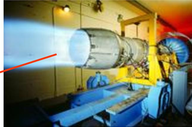
***Sensors are needed for real-time monitoring of temperature, stress, fuel blow out, combustion instabilities, noise and NO<sub>x</sub> emission etc.***
