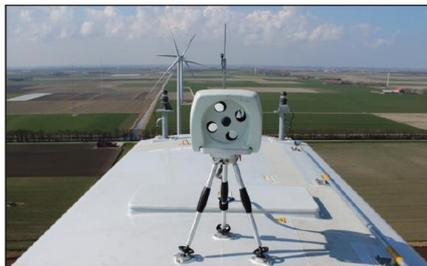
Nacelle Mounted Lidar – \$80k to \$100k per sensor
